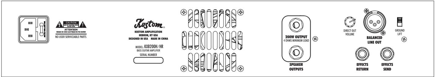
**Speaker Outputs:** These are two-conductor, ¼-inch external speaker jacks. These jacks are wired in a parallel configuration. Use them to connect the amplifier head to speaker cabinets with a minimum total impedance of 4 ohms. **(Note:** Be sure that the amp is turned off before connecting or disconnecting speaker cabinets.)
