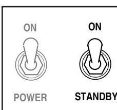
Wait at least 30 seconds and then flip the **STANDBY** switch to the ON position. This prevents tube problems and increases their toneful life substantially.
