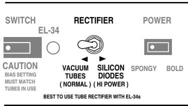
**SOLID STATE: (Hi Power)** calls up the silicone diode rectifiers which offer more punch, a tighter attack with added brightness and substantially more headroom. This would be the preferred position for loud clean playing or tight rhythmic playing with a high front end GAIN setting.
