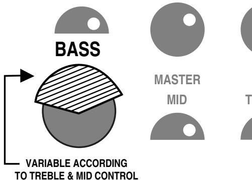
For the most balanced sound and a balance of power between the three rotary tone controls, try to use the **TREBLE** Control in its middle ranges. This scenario produces nearly equal representation of all the frequencies on the tone controls and provides a great neutral starting point for further tweaking.
