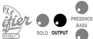
**NOTE:** When using the **EFFECTS RETURN** as an input - to use the *Recto* as a power amp - the **SOLO** Control can be used to attain a footswitchable boost if the Footswitch is connected. It is wired in parallel to the **OUTPUT** Control and therefore also controls the volume of the power section.
