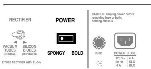
Using either *Rectifier* Solo Head in this power setting will also extend tube life and overall reliability, while still producing enough to work many of your gigs...and all of your recording needs!
