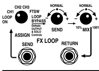
**NOTE:** **LOOP BYPASS** defeats the Front Panel **OUTPUT** and **SOLO** Controls as they are part of the **FX RETURN** circuit. This tube stage and associated circuitry are omitted when you select **LOOP BYPASS**. The Channel MASTER Controls become the final output controls in this case.
