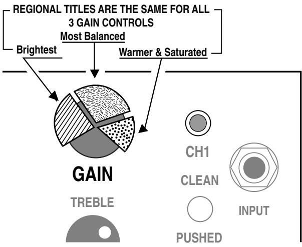
To simplify the **GAIN** Controls' role in shaping the overall tone of the sound we will look at it in two ways - 1; alone and 2; in conjunction with the tone controls.
