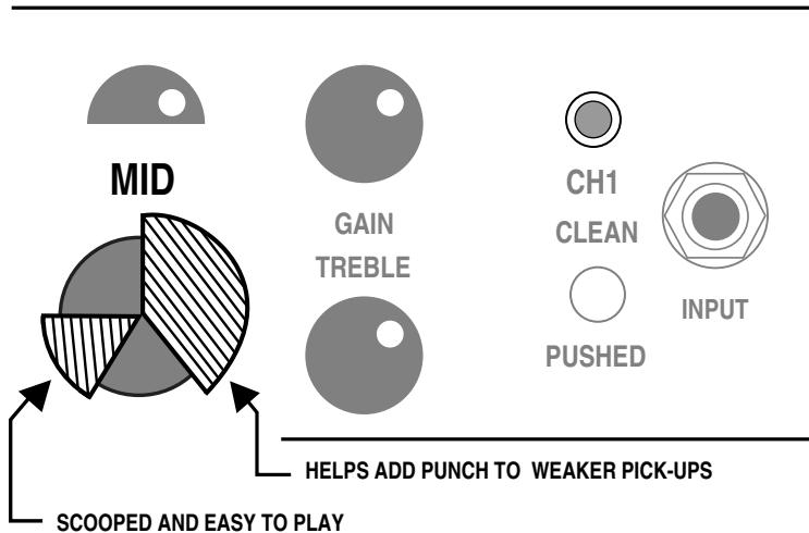
in the room. While these **MIDDLE** Control settings (2:00 - 5:00) can introduce added gain and create enhanced focus, the trade-off will be a stiffer, more forward, less compressed feel.
