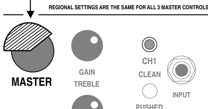
Again, we suggest using the **MASTER** Control in its *sensible* ranges (9:00 - 2:00). Here, the channels will be easier to match with each other and the Effects Loop will see more reasonable signal levels.
