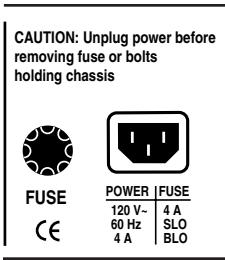
If you see nothing abnormal as you lift the STANDBY switch, it is possible that a power tube shorted temporarily and blew the Fuse. If this is the case it may work again normally. To be safe, you might want to replace just the adjacent tube or all power tubes in the "shotgun" troubleshooting tradition and save the replaced set as spares. Spare fuses are a must for the fabled cord bag along with your spare tubes. Always carry both for they could be worth their weight in gold someday.
