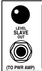
**NOTE:** Once a signal is taken from the **SLAVE**, it can not be inserted back into the **FX Loop Return** jack or a feedback loop will occur. Much like holding a microphone into the PA system's cabinets...a loud high pitched squeal will be the result.
