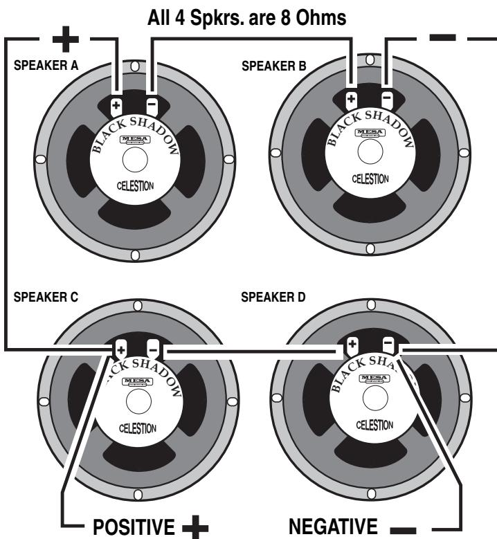
Simply connect the Positive side of Speaker A to the Positive side of Speaker C.
